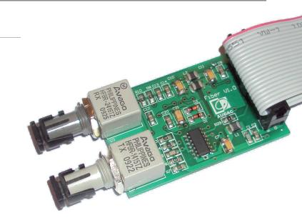
The R2OPT is a fiber interconnection interface for the R2 and M2 Digital Multi-Zone Matrix Systems.
