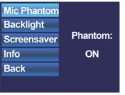
With the "Mic Phantom" option, the 15V DC phantom power to the microphone input on the wall panel can be enabled and disabled, while the "Backlight" option enables you to adjust the backlight intensity for the LCD display. With the "Screensaver" option, the desired screensaver and the time before the sceensaver shows up can be set. Info shows some more information about the wallpanel and the current software version.
