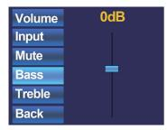
The latest settings which can be changed to the zones are the two band tone control. The tone control can be activated by selecting the "Bass" and "Treble" buttons, and the adjustment of the tone control works with a fader just as the volume control. You can increase and decrease the high and low tones the same way as adjusting the volume, by simply rotating the selection dial. The Bass and Treble both can be adjusted between the ranges of +9dB and -9dB.
