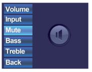
When the input selection is made, you can scroll further through the settings menu and make other changes such as muting, and changing the tone control. When the zone should be muted, just scroll to the "Mute button" and push the selection dial. When the selection dial is pushed, there will be toggled between "Mute" and "Unmute".
