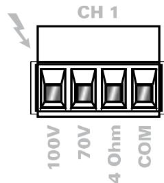
The table below shows the impedance and output voltage for each power tap.
